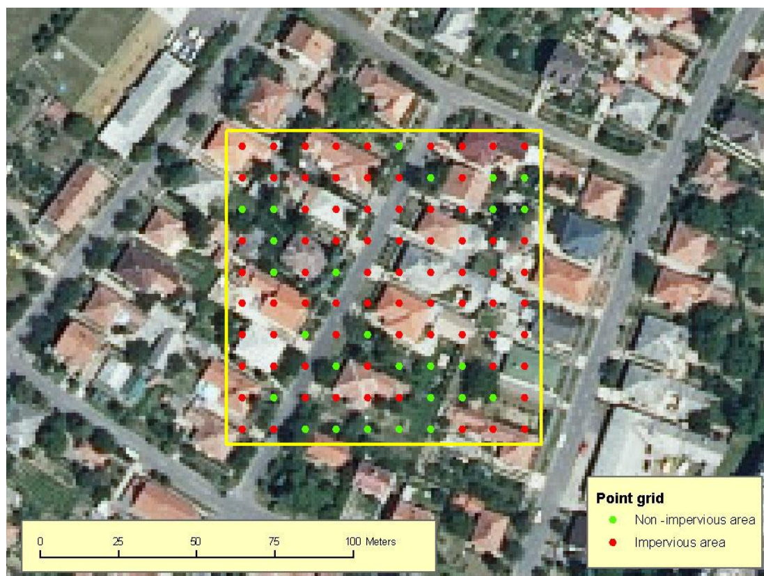
Figure 2 Validation methodology of European SSE data. By counting the number of impervious points inside the 100x100 m grid cell (total of 100 points), the interpreter estimates sealing degree of the sample cell 18 .
